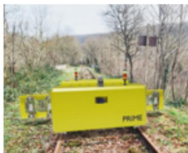
The robot PRIME equipped with its new vegetation control accessory.
