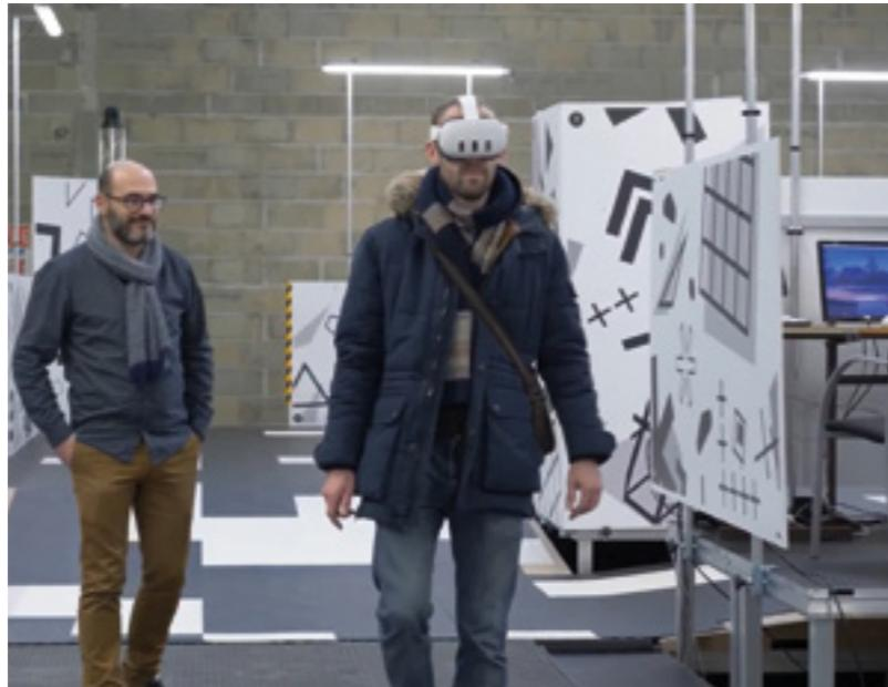
The virtual reality platform is synchronized with a physical environment, and various scenarios are proposed to test subjects equipped with headsets.
