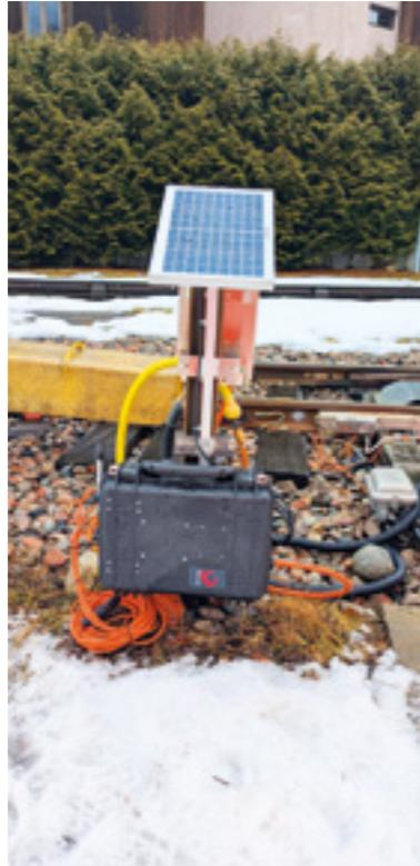
This prototype of REG'GAZ, which is designed to prevent snow accumulation and frost formation on track switches, is testing temperature regulation.
